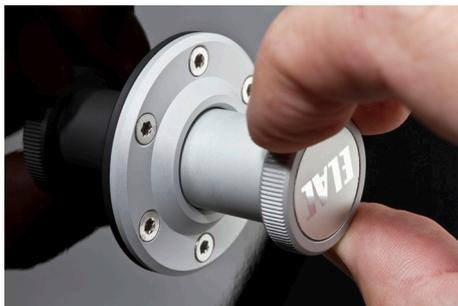
By means of an adjusting knob at the rear side of the speaker the whole VX-JET driver may be moved 8 mm out (in front of the baffle) or 8 mm in (behind the baffle). The idea behind is the fact that each room has its own acoustical behaviour and the same speaker produces different sounds in different rooms. The wish of “one speaker for all rooms” has
